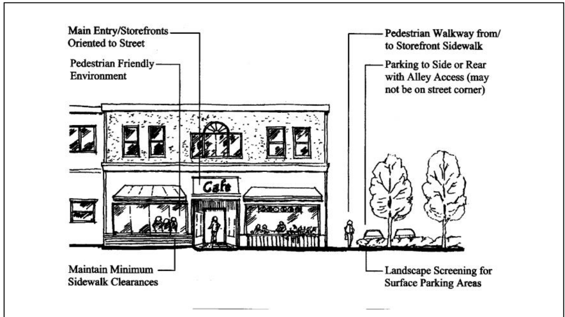
Figure 2.2.140D - Building Orientation (Typical)
